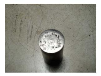
This is the acid eroded surface of a tappet showing the disintegration of the face where it rides on the cam.
